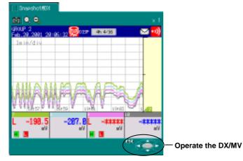
You can also double-click the image data file (.png) of the screen that was created by the DX/MV to display the snapshot folder, but you cannot operate the DX/MV.
